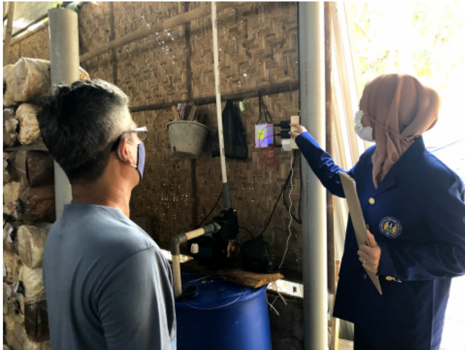
Figure 1. Students demonstrate an IoT device for monitoring the temperature and humidity of an oyster mushroom barn. A DHT sensor is placed inside the barn, connected to a NodeMCU ESP8266 microcontroller that sends data to a smartphone app in real time.
