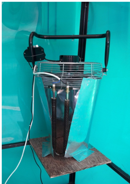
Figure 5. Heater and Fan
