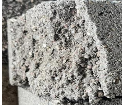
Picture 5 Field specimen cavity
