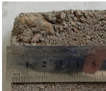
Picture 3 Fine aggregates in field test specimens
