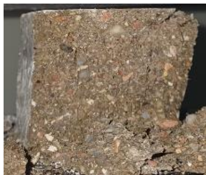
Picture 4 Cavity density of laboratory test pieces
