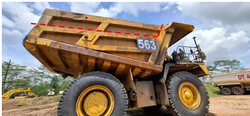
Figure 8 Illustration of Cutting the Mud Body Patria vessel
