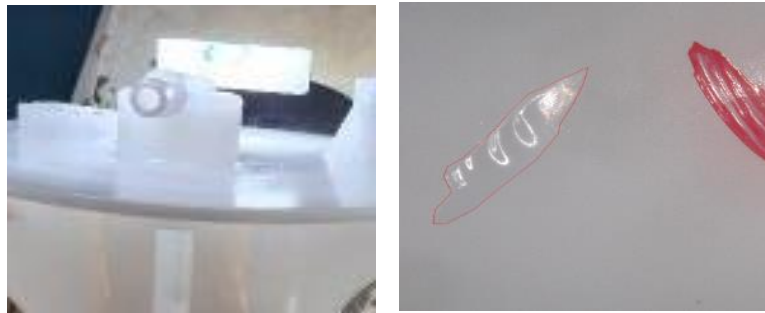
Figure 1 Delamination defects in breather pipe flange products
