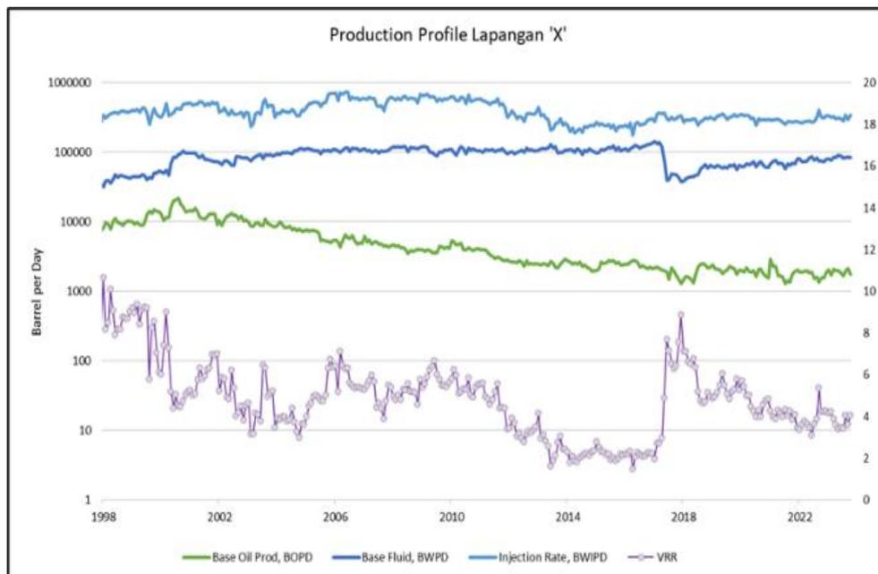
**Figure 1 VRR Graph on Field Production and Injection**
