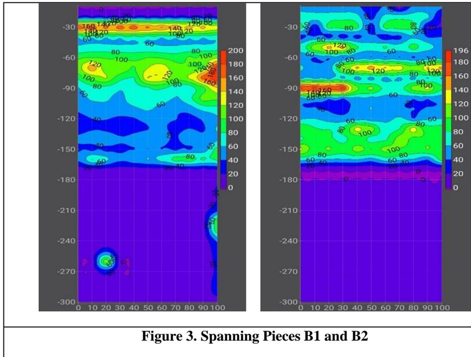
The acquisition of Stretches 1 and 2 based on the results of geoelectric testing in the barracks staff housing produced subsurface data as shown in the figure above. In stretch 1 there is a free aquifer with a small volume. Depressed aquifers can be found at depths of  $\pm 160 - 300$  m.
