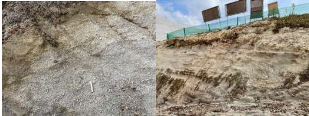
Figure 7 Unit outcrop conditions per interlude of fine tuff and coarse tuff (Observation of Margatiga Dam Work, 2021)
